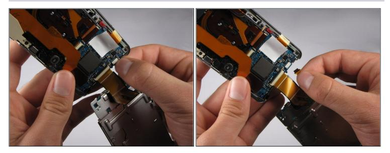
• Disconnect the small ribbon-wire by gently pulling on the small ribbon-wire where it connects with the motherboard.
