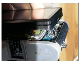
Place a plastic opening tool into the gap between the back panel and camera body, from both the top and the bottom of camera. Carefully pry open the camera and separate the back panel.
