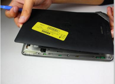
Pry off the back cover with the plastic opening tool. Go around the device with the tool to ensure complete detachment.
