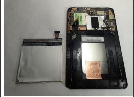
Using a spudger carefully pry the battery up. It is glued down so slight pressure may be needed.
