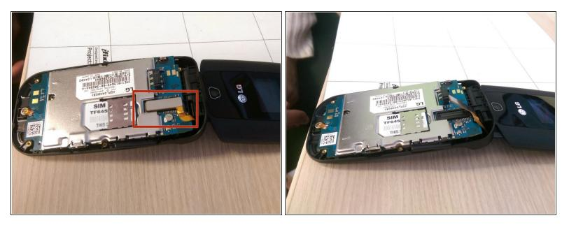
Use the plastic opening tool or fingernail to lift the rectangular piece up. The piece can be identified by the orange tape attached to it.
