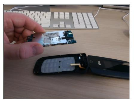
• Remove the logic board by lifting up.
