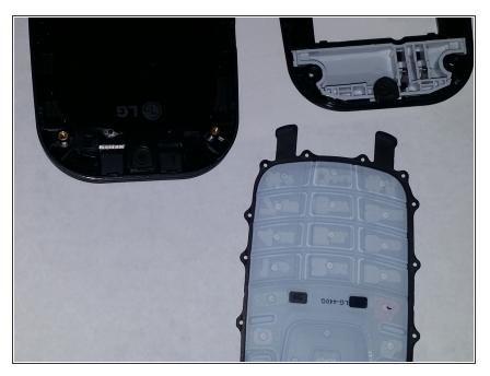
• Remove the keypad from the phone by pushing the keypad itself out from the front of the phone. Then, lift the keypad out of the casing to separate the keypad from the casing.
