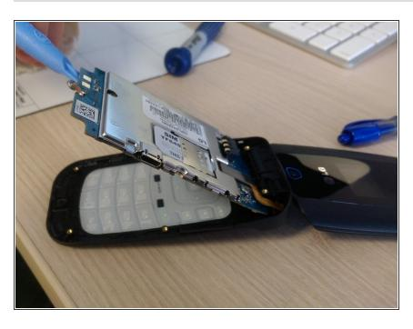
Dislodge the logic board using a plastic opening tool.
