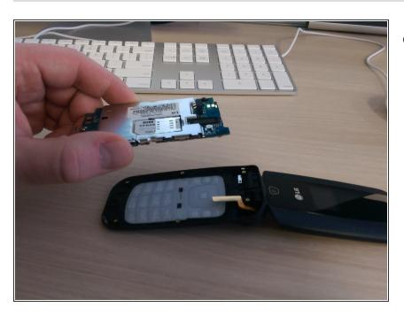
Remove the logic board by lifting up.
