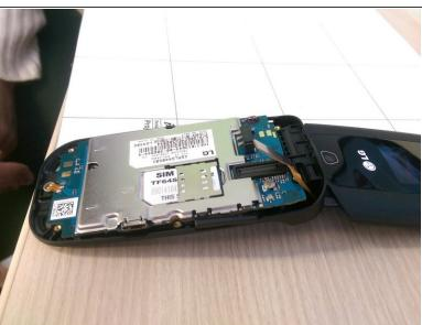
Use the plastic opening tool or fingernail to lift the rectangular piece up. The piece can be identified by the orange tape attached to it.
