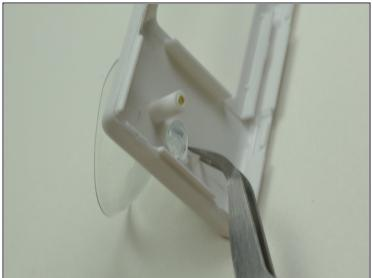
• Using <u>tweezers</u>, push the edges of the back end of the suction cup inward.
