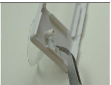
Using tweezers, push the edges of the back end of the suction cup inward.
