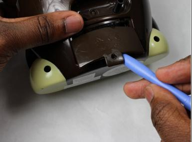
• Use the plastic opening tool to pry up the battery compartment cover.
