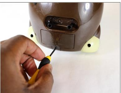
Use the Phillips #00 screwdriver to loosen the 6.8 mm screw.
