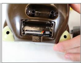
Once compartment is open, remove the two AAA batteries.
