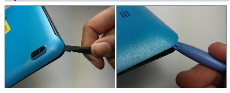
Pry off the backplate by inserting a spudger or plastic opening tool into each corner and popping them open.
