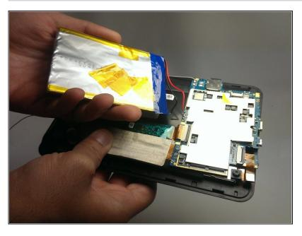
• Fully remove the battery from the device.
