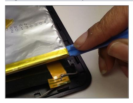
Un-stick the battery from the motherboard assembly with the plastic opening tool.
