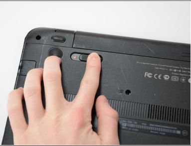
Carefully slide the leftmost switch to the right, which is the unlock position, as shown by the orange unlock icon.
