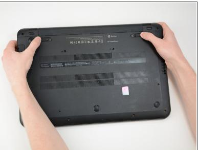
Flip the laptop over and locate the release switches located at the back corners of the laptop.
