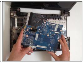
Carefully pick up the Mother board and disconnect the Battery cable.
