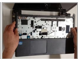
Carefully separate the upper cover and remove it.
