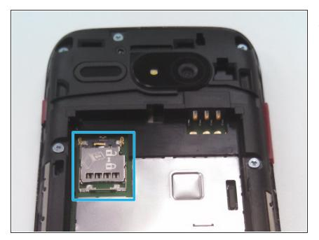
The SIM card slot can be seen in the middle left of the photograph.
