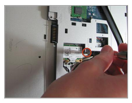
Remove the single 5mm screw that connects the keyboard to the palm assembly with the Phillips head screwdriver.
