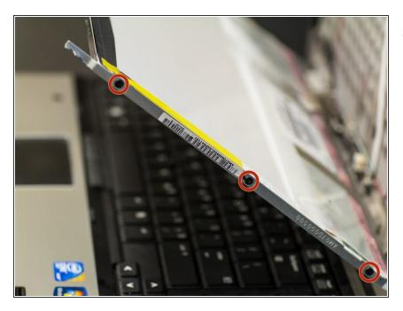
• Remove the three PH0 screws from each side of the LCD assembly.
