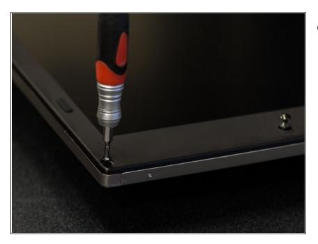
• Screw in the four corner PH0 screws
