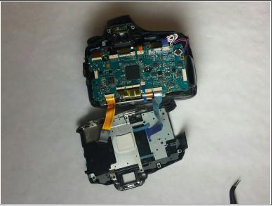
Once all of the screws are out, open the camera as shown in the picture.
