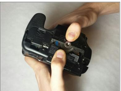
Unscrew every screw on the side and back camera to pry open the back plastic portion of the camera. The screws will be 2.1mm and 1.5mm.
