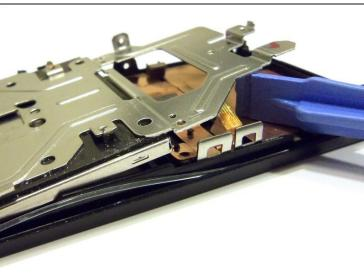
• Pry the end of the screen with the plastic opening tool.
