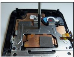
Use Phillips size 00 and remove the 3 screws as shown.
