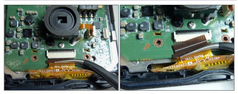
• Use tweezers to grab the wire ribbon, then pull the wire out of connection.
