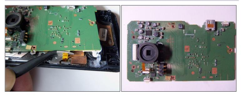
• Use tweezers to disconnect the wire as shown. This will loosen the motherboard from the rear case.
