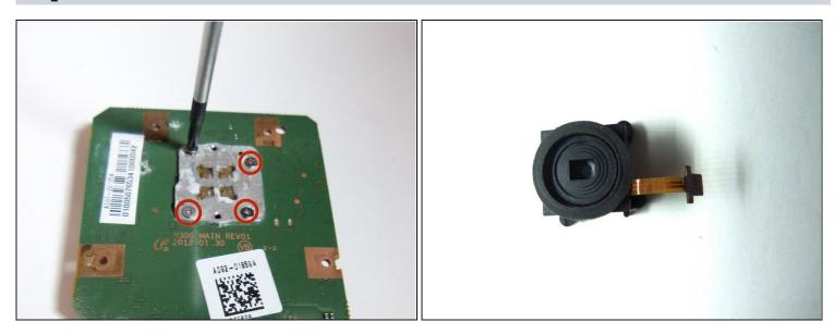
• Remove all 4 PH(00) screws, this will loosen the lens from the motherboard.
