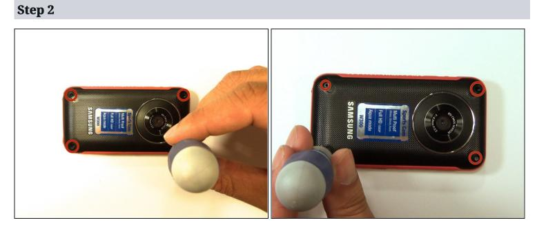
• Remove four screws with a Hex 1.5 mm screwdriver.
