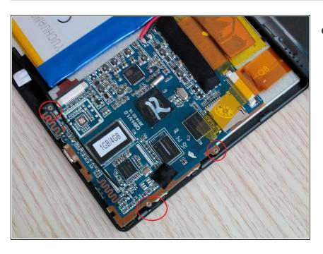
remove the screws of the main board.
