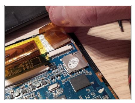
remove the third connecor, it is next to the connecotr in step 3.
