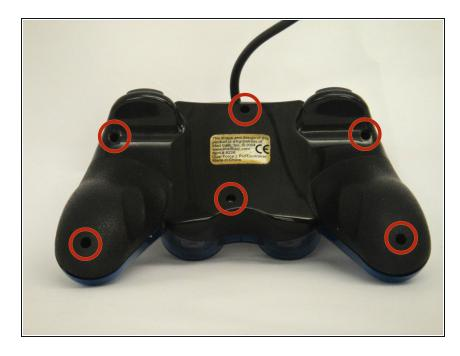
Using the Phillips #1 screwdriver, remove the six 7 mm screws from the rear cover.
