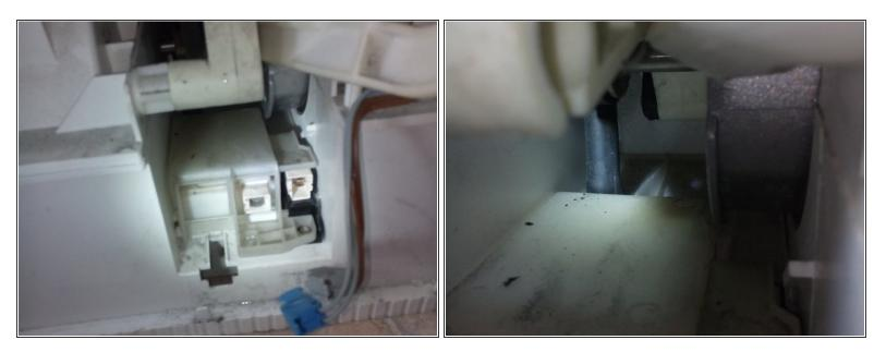
Remove the cable from the float and the pump and pull off the hose at the back. The motor can be folded upwards.
