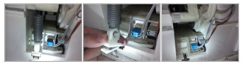
• After removing the side cover (if you are standing in front of it on the right) the motor of the drum becomes visible. The pump of the condensation water tank and the float are located directly underneath. The drive tensioner must be loosened for removal/exchange.
