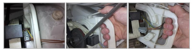
• Remove all plugs from the drive (not shown in the picture!) and remove the placeholder. Unlock the lock with your thumb.
