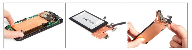
• Remove the battery with card reader assembly together at first. And then separate them. The battery flex is stuck on the back of the card reader assembly.
