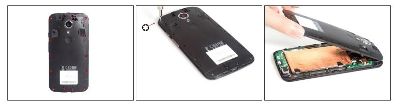
• Unscrew 14 screws and remove the back frame.
