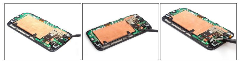
Release SIM & SD card reader assembly connector and battery connector. Get loosen the vibrator.
