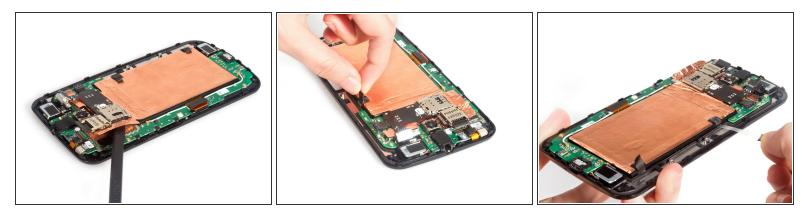
• Loosen kinds of stickers fastening card reader assembly and battery.
