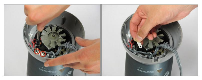
• With the Phillips head #2 screwdriver, remove the two 10mm screws that secure the white bracket.
