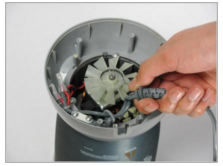
• Gently lift the power cord from its side slot and place it to the side.
