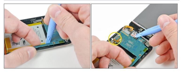
• Use an iPod opening tool to slightly lift the edge of the logic board next to the battery enough to grab it with your other hand.
