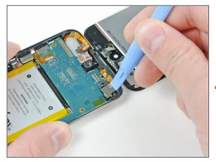
• Use the edge of an iPod opening tool to gently pry, but not remove, the rear-facing camera away from the rear case.
