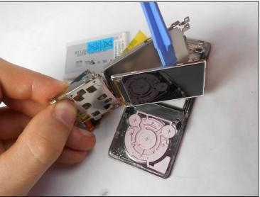
• Use a plastic opening tool to remove the screen from metal back plate.
