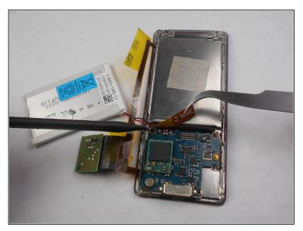
Remove screen connection from motherboard using tweezers and spudger.
