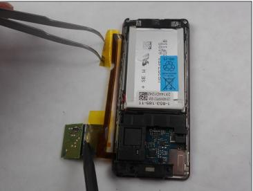
• Peel back the layer of tape along with the processor, which is located just below the battery, using the <u>tweezers</u> and the spudger.
