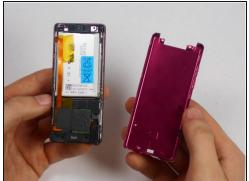
Remove the back plate from the device.
