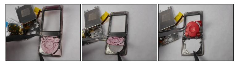
Remove buttons from front display panel by pushing button display from the front of the device
