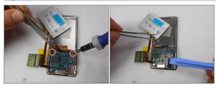
• Use a Phillips #00 screwdriver to unscrew two 2 mm screws, and remove the motherboard from the device with tweezers and a plastic opening tool.
