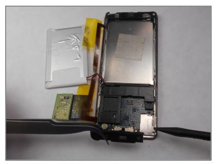
Use a nylon spudger or tweezers to remove the plastic USB cover.
