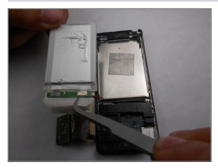
Remove the stickers from the battery terminals, which are on the underside of the battery.
