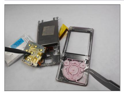
Ensure that button connection is completely separated from the buttons.
