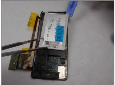
• Slide a prying tool underneath the top portion of the battery and lift it from the case.
