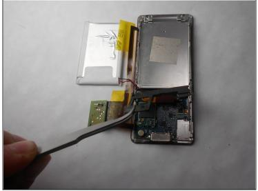
Remove the plastic protective frame located over the motherboard with tweezers and a spudger.
