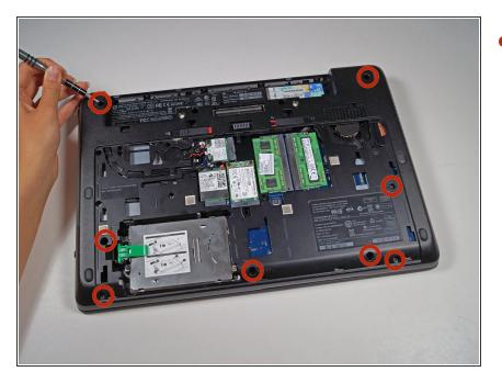
Remove the eight 6mm screws with a T8 Torx screwdriver.
