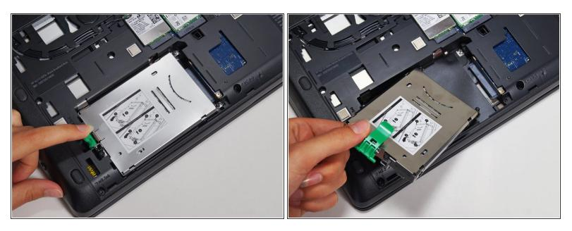
• Pull the green tab away from the metal casing and lift the drive out.
