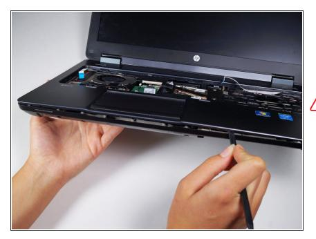
There are still ribbons that need to be removed before the top cover separates completely; do not yank
