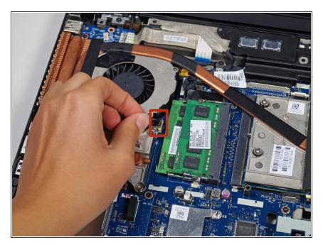
Gently pull up on the 4 pin fan power connector cable to unplug it from the system.
