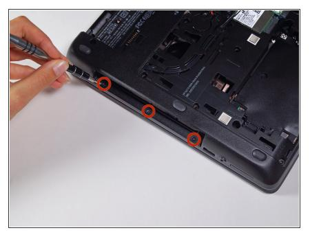
Remove three more 4mm screws from the optical drive compartment with a T8 Torx screwdriver.
