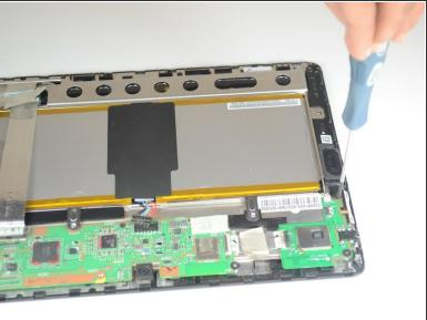
Remove the four 2 mm Phillips #00 screws holding the battery tray in place.
