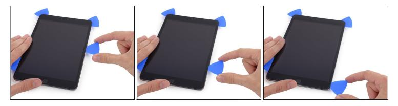
• Continue to slide the pick down the right edge of the iPad, releasing the adhesive.
