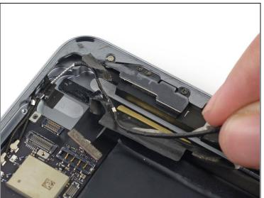
Pull the antenna cable out from under the corner of the right speaker.
