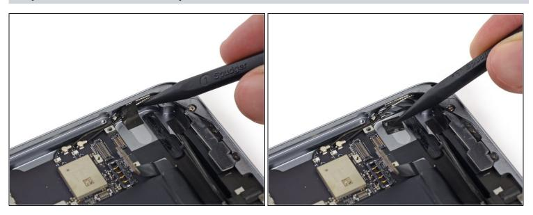
• Use the tip of a spudger to peel the tape off of the antenna cables near the logic board.
