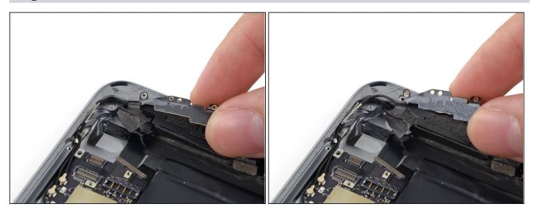
• Pull the bend of the antenna cable out of the corner of the case.
