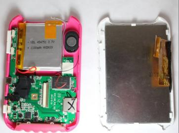
• Locate the light grey clamp on the motherboard and gently use two index fingers to disconnect the black LCD cable from the motherboard.
