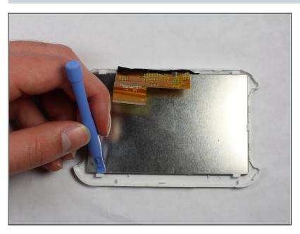
Gently press on the white clamp using the blue spudger to remove the metal panel.
