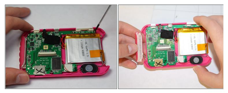
• If you need to remove the back part of the casing, after disconnecting the LCD display from the motherboard, remove the screws holding down the motherboard. Remove the plastic power and volume buttons. remove the two side grips of the device.
