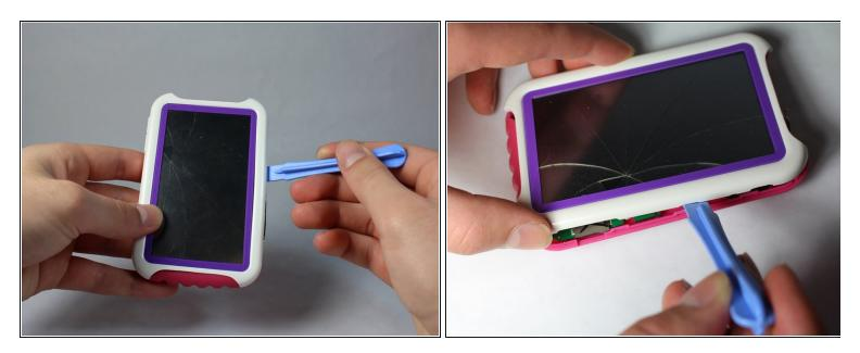
• Use a spudger to pry open the case of your device to reveal the inside.
