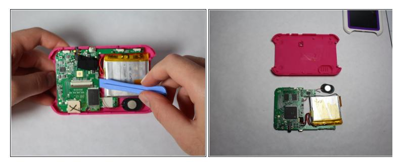
Remove the motherboard, speaker, and battery as a whole, which leaves just the back casing
