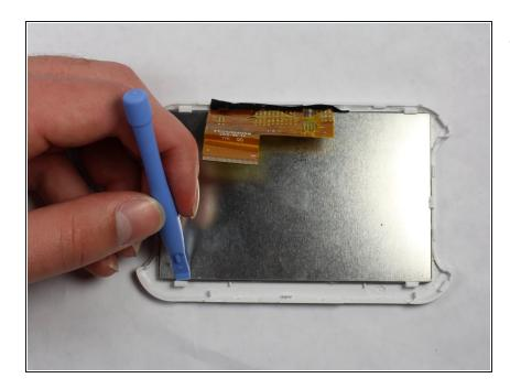
• Use the spudger to pry the LCD from the clamps holding it to the case.
