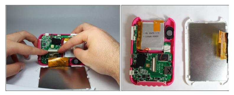
• Disconnect the LCD cable from the motherboard by pressing together the two sides of the clamp to separate the device into two.
