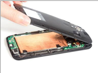
Remove back frame. Be sure to remember where the screws go; they are different sizes
