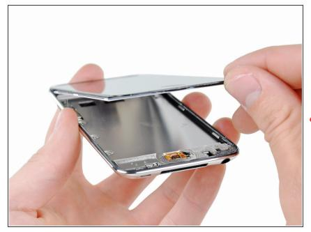
When there is enough room to grab the bottom edge of the front panel, lift it away from the body of the Touch to peel up the adhesive along its left and right edges.
