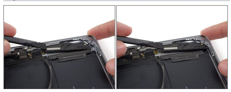
• Push from the Lightning connector end with the flat end of a spudger to free the speaker from the lip of the rear case.
