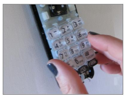
Gently remove the loose keyboard from the lined gel casing located under the front housing of the front of the phone.
