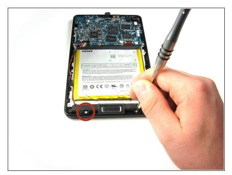
Unscrew the two 3.5mm T5 Torx screws at the base of the speaker.
