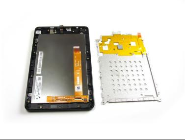
Remove the metal plate from the device.
