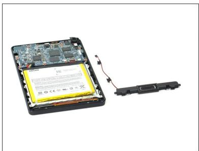
Lift the speaker out of the device.
