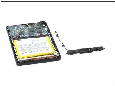
Lift the speaker out of the device.
