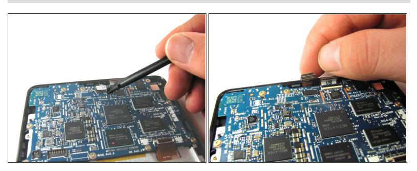
Disconnect the black and white connector at the very top-center of the motherboard by unclipping it using the flat side of the spudger.
