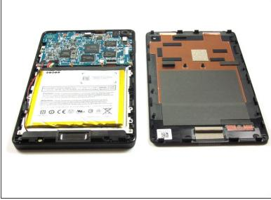
Carefully separate the back panel from the rest of the device internals.
