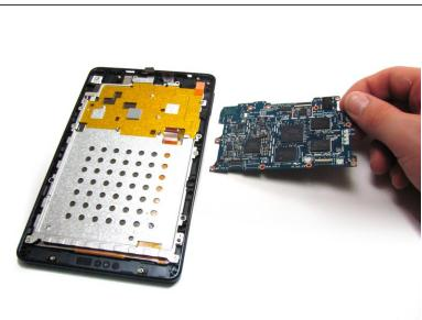
Starting from the bottom, lift the motherboard out of the device. You will have to push the motherboard about two millimeters toward the top of the device to unhook the top edge.
