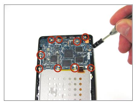
Unscrew the ten 3.5mm T5 Torx screws around the edge of the motherboard.
