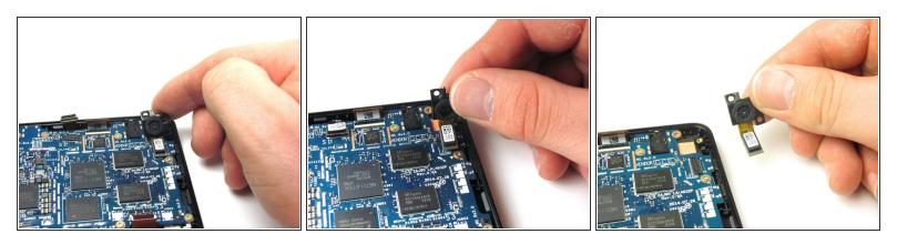
A Be careful not to damage the camera lens as you remove the camera.
