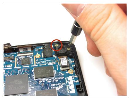
• Unscrew the two 3.5mm T5 Torx Screws from the top of the camera.
