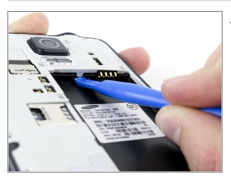
Use a plastic opening tool to loosen the clasps around the battery housing.
