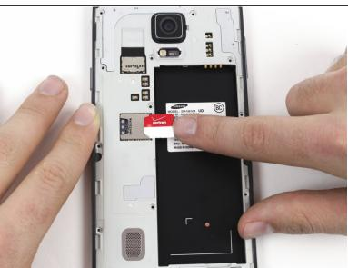
Remove the SIM card by first pushing the card slightly out of its housing, then pulling it the rest of the way.
