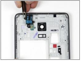
Use the plastic spudger and tweezers to remove the headphone jack from the middle housing.
