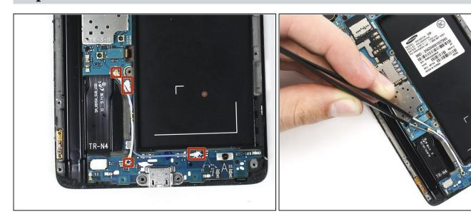
• Use a set of <u>tweezers</u> to remove the two antenna cables.
