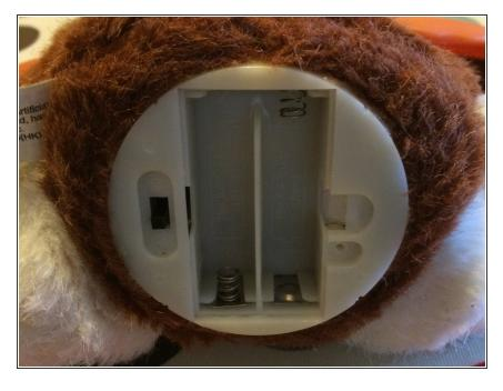
Toys with motors of this kind need the batteries to be good and strong before they'll dance. So before you open Gizmo up, give him a fresh pair of alkaline AA batteries. Like most toys, his battery compartment is attached with a single 00 Phillips screw.
