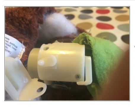
• Although I think that most of these toys will break in exactly the way mine did, your problem might be different. The head controller has a circular fixing that slips over a knob on the base, a part screwed into the other side, and a groove that takes the rotating button to create the movement.
