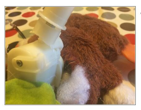
Gizmo has a simple motor linking his head and body. It's covered with a green cover which is attached with not very strong adhesive. Pull it off to get at the workings. You can see that in my Gizmo, the plastic piece that links the head and body had broken.
