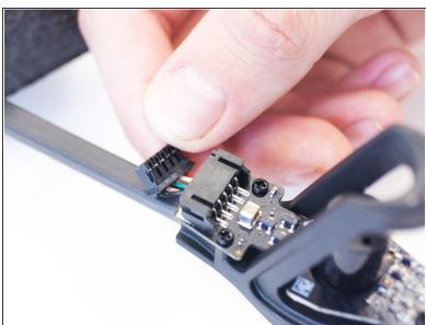
Disconnect the connector at the bottom of the motor assembly.
