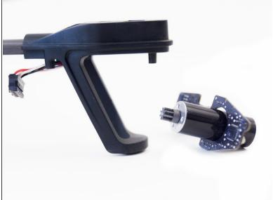
Carefully wiggle out the motor assembly out of the arm.
