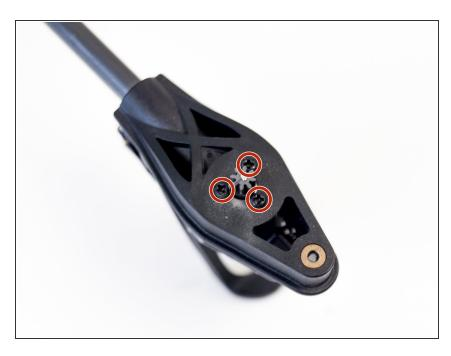
Remove the three 5mm screws on the top of the motor assembly with a PH00 bit.
