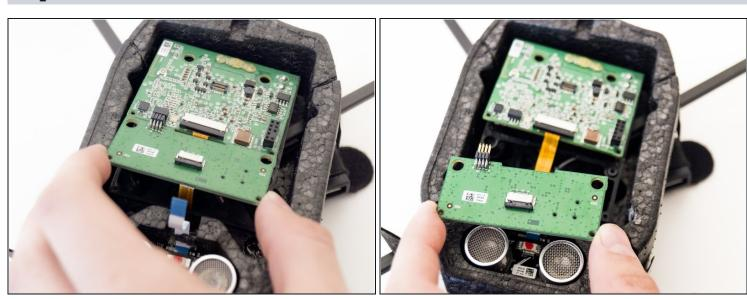
• Carefully pull the secondary board from the mainboard.
