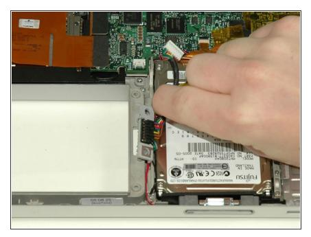
Lift the battery connector out of the computer, removing tape as necessary.
