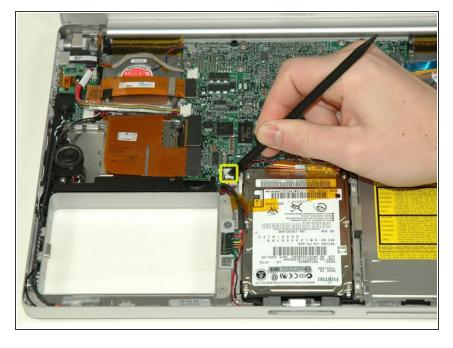
Disconnect the sleep light cable from the logic board to gain access to the battery connector cable beneath it.
