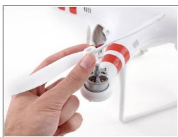
• Gently press down the motor shaft and lift the propeller up to remove it.
