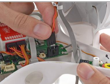
Lift the GPS cable molex connector up out of its socket on the main board.
