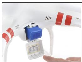
Press down on battery door release tab to flip the battery door open.
