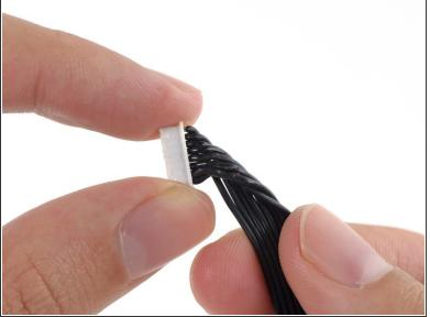
Twist the other end of the G8 cable molex connector as shown in order to plug in the H3-2D gimbal.
