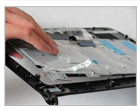
Slowly separate the main part of the keyboard from the metal plate by pressing firmly on the key side of the keyboard and lifting from the back side.
