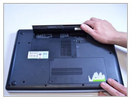
• Carefully remove the battery from its compartment.
