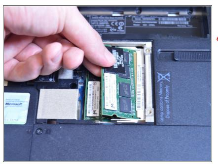
• Carefully remove module from slot.
