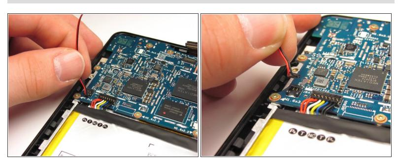
• Unclip the speaker wire that runs up the side of the battery and clips into the motherboard next to the battery connector. Gently pull it straight up.
