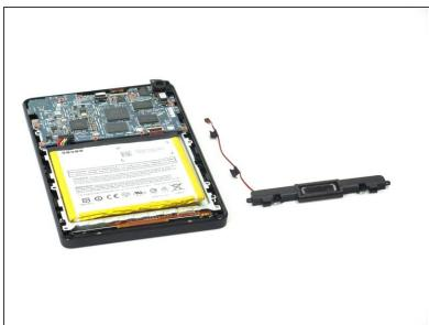
Lift the speaker out of the device.
