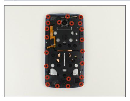
Remove the twenty-two 2.3 mm T3 Torx screws with the T3 Torx Screwdriver.
