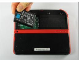
Remove the battery from its housing by lifting it up from the side closest to the outside edge.
