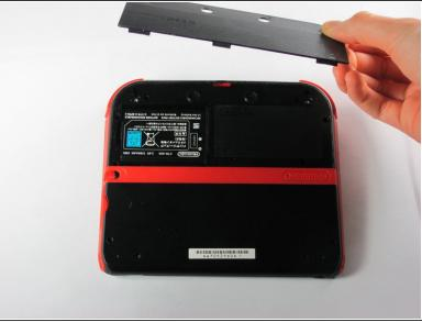
Hinge the upper rear panel upwards and outwards to remove it.
